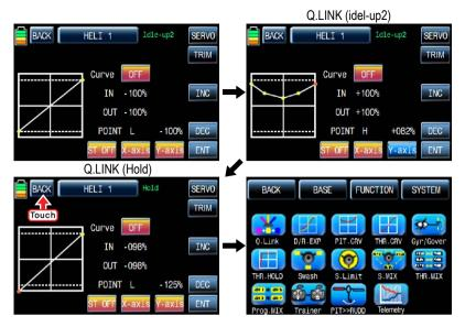
If you touch OFF icon in Curve line, it is switched to ON and the operation curve is smoother. After setup, touch "TRIM" icon in the top right to call the pitch, throttle curve trim setup page.
