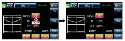
In the pitch, throttle curve trim setup page, you may designate the pitch, throttle curve control with DV1, DV2, DV3, DV4, SL1 and SL2 so that you can control servo movement with throttle curve control such as the hovering in normal Q.Link and IDLE 1, IDEL 2 Q.Link.
