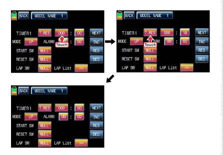
Touch the value in "MODE" line to select "UP" or "DOWN". Timer may be counted down or counted up with your choice. Count-up timer is to count from zero to the setup time and Countdown timer is to count from the setup time to zero.
