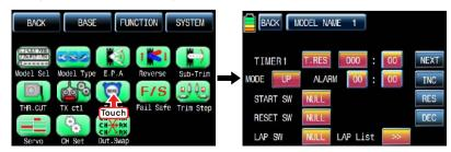
Timer consists of TIMER1 and TIMER2. The flight data is saved to SD card on transmitter during the flight time is operating in TIMER1 mode but TIMER2 don't have the storing function for the flight data.
