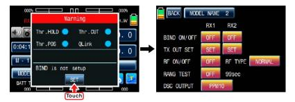
After accessing to Tx ctl(BIND), Turn on receiver's power and press & hold Bind button on receiver for over 3 sec to enter binding mode. Touch OFF icon to switch to ON, which is in the cross line of BIND ON/OFF and RX1 then the system has been connected. If the binding process has failed, repeat the whole procedure.
