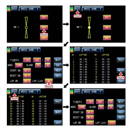
Touch "NEXT" icon on the right in Timer 1 setup page, you may call Timer 2 setup page. You are able to set Timer 2 as the same as explained above. Timer 2 don't have the function of the flight data saving so it can calculate the time only.
