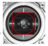
The Swash rotation function in the bottom is used to make the swash that mz-24 doesn't support available by rotating the swash angle
