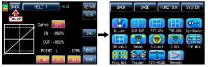
If you touch OFF icon in Curve line, it is changed to ON and the operation curve is smoother. You may set the pitch, throttle curve trim by touching "TRIM" icon in the top right. The setup method is explained at PIT.CRV
