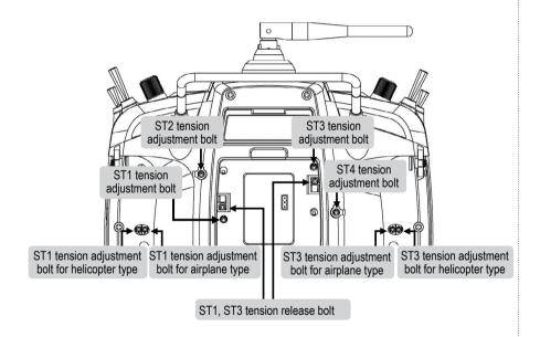
You may release the stick tension with ST1 or ST3 tension release bolts. Turn the bolts clockwise then the stick tension is released
