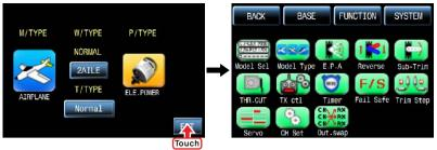
"Wizard setup" is used to set the basic function of a model and the essential function of flight one by one. Please refer to the example of helicopter type as below.
