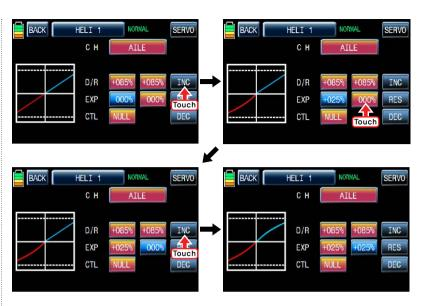
After "D/R", "EXP" setup, perform CTL setup. It is used to assign the switch to D/R, EXP function
