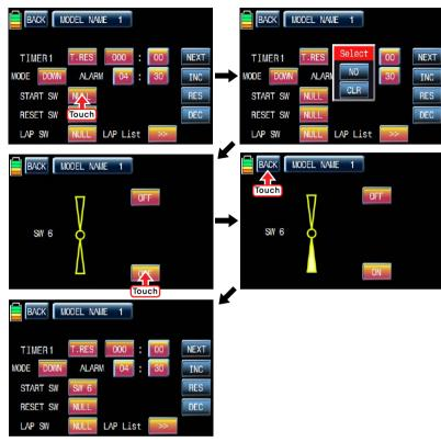
When START SW setup is completed, you may set RESET SW function. Touch the "NULL" icon in "RESET SW" to call "select" message popup. Now, move the switch with your choice then this switch is set to on/ off switch for "RESET SW" and the switch direction setup page appears. You may change ON/OFF by touching icons. When the switch is moved to the direction of ON, the function is operated. Touch "Back" icon to return TIMER setup page
