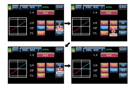
After "D/R", "EXP" setup, perform CTL setup. It is used to assign the switch to D/R, EXP function
