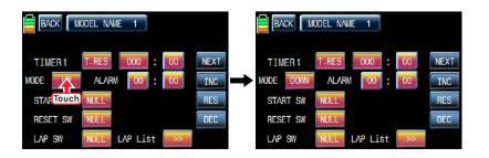
After "MODE" setup, you need to set "ALARM". The alarm sounds from the last 20 seconds in the setup time. The first 10 seconds, it sounds at intervals of 2 seconds and the next 10 seconds, it sounds at interval of 1 second
